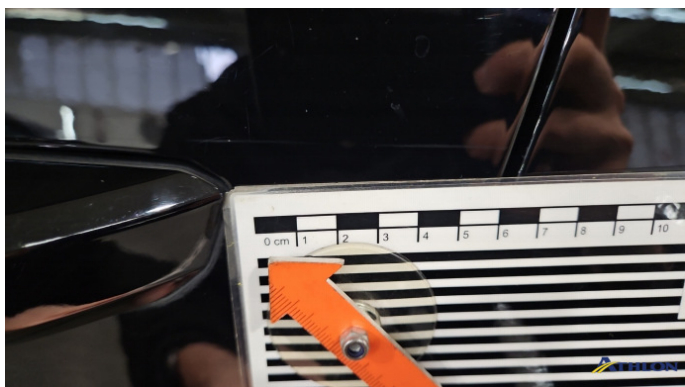
7. Tür Hinten - Links Kratzer
